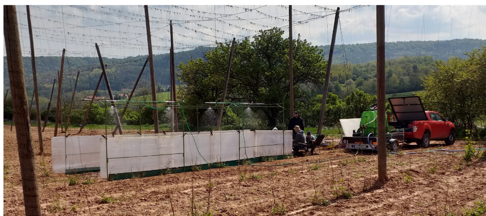
Figure 3: Rainfall simulator in hop garden (end of cropstage period 1). Source: Photo taken by the authors.
