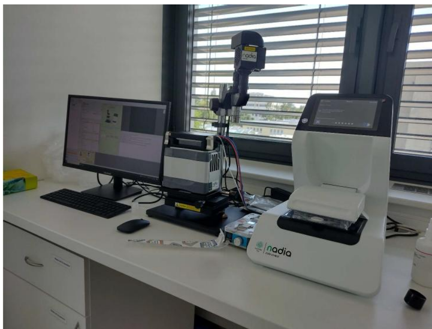
Microfluidic system for cell encapsulation, acquired under Specific Objective B (Faculty of Science). Photo: Faculty of Science, USB
